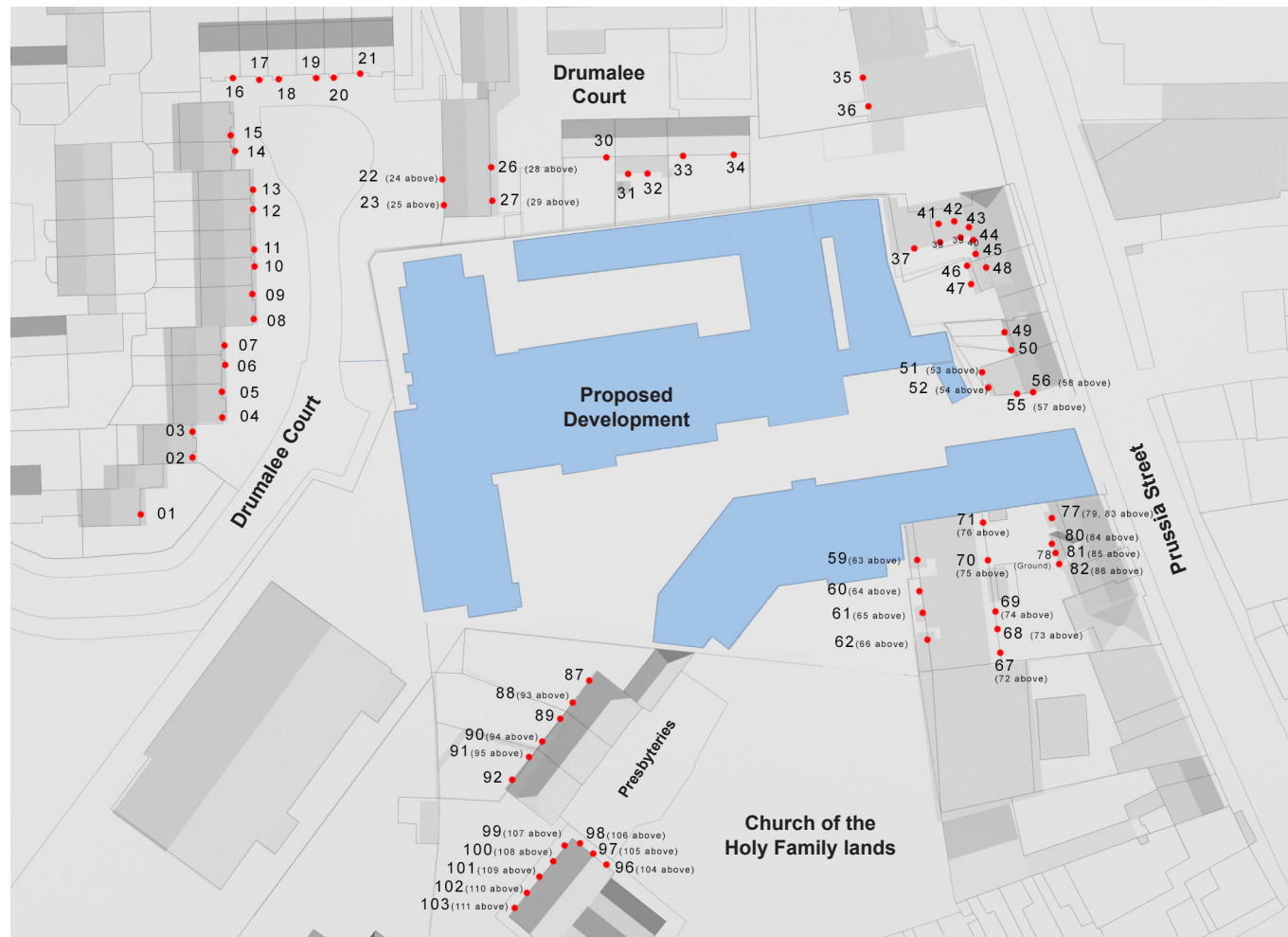
Figure 3.1: Indicative diagram showing location of sample windows (red dots) assessed as part of this analysis
