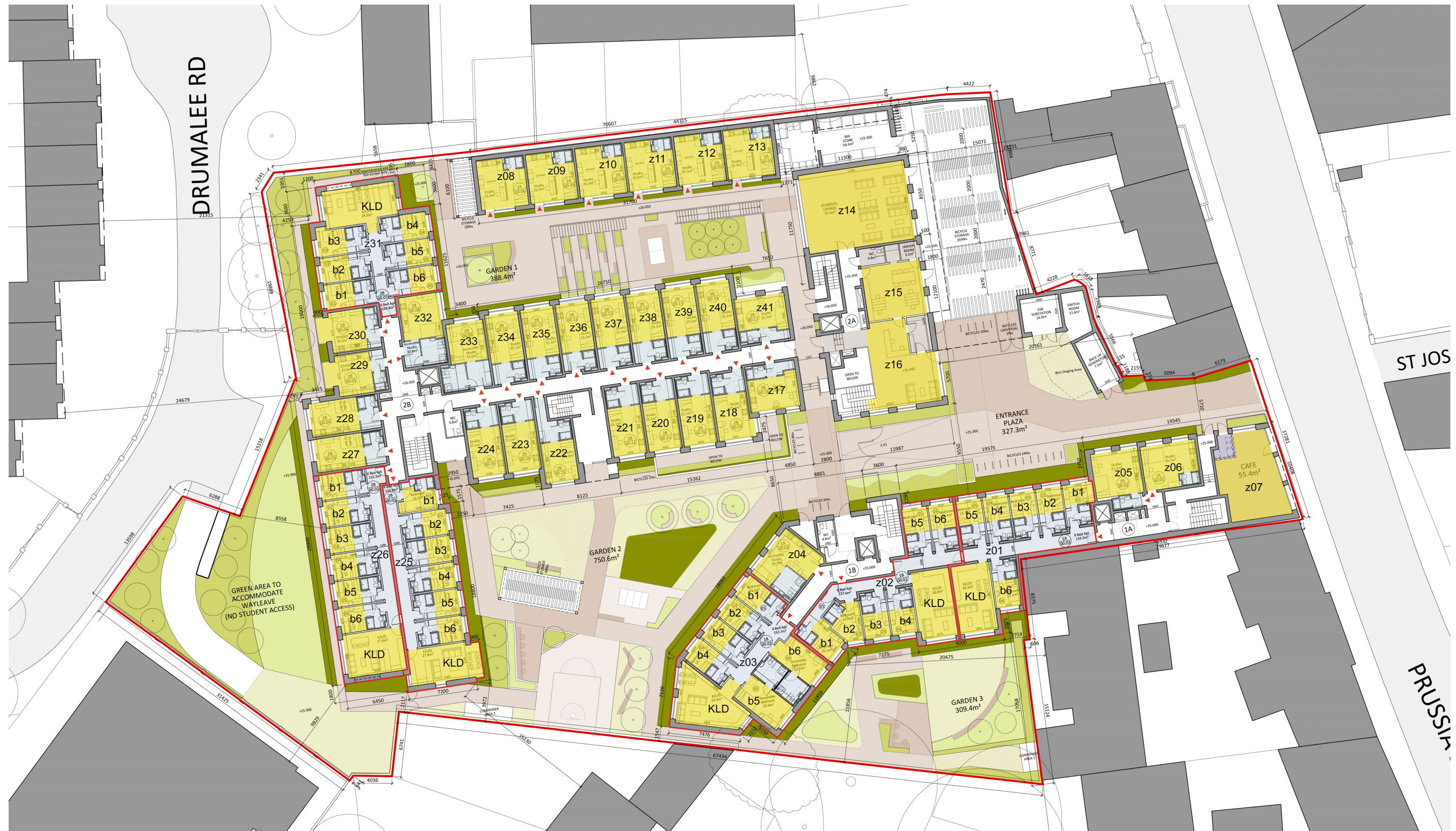
Figure 4.1: Indicative diagram based on the proposed Floor 00 plan prepared by O'Mahony Pike Architects (not to scale) showing the location of rooms assessed as part of this analysis
